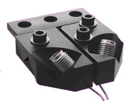
The **DUAL MICROWAVE PROBE** consists of two separate probes mounted on a single holder. One probe is fixed to the holder; the other is adjustable. Each probe may be individually configured with GSG, GS, or SG footprints. The probe to probe (signal to signal) spacing is user adjustable over a 4000 micron (160 mil) range. When ordering, an initial setting (up to .75 inches) should be specified. The spacing is measured as the distance between the signal contacts of each probe.
