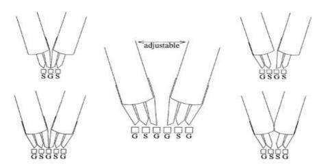
Microwave probes with frequencies up to 110GHz are available. Choose from either the Model 40A (2.9mm connector), Model 50A (2.4mm connector) Model 67A (1.85mm connector) or the Model 110H (1.0mm connector).
